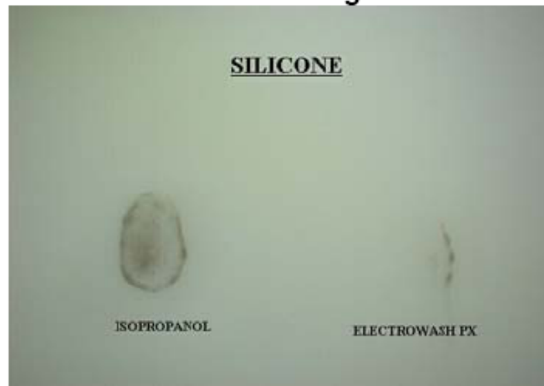
Soil after cleaning
