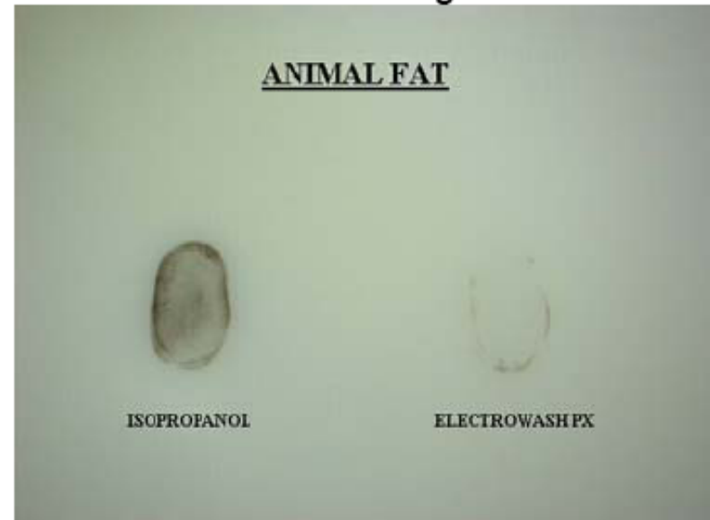
Soil after cleaning
