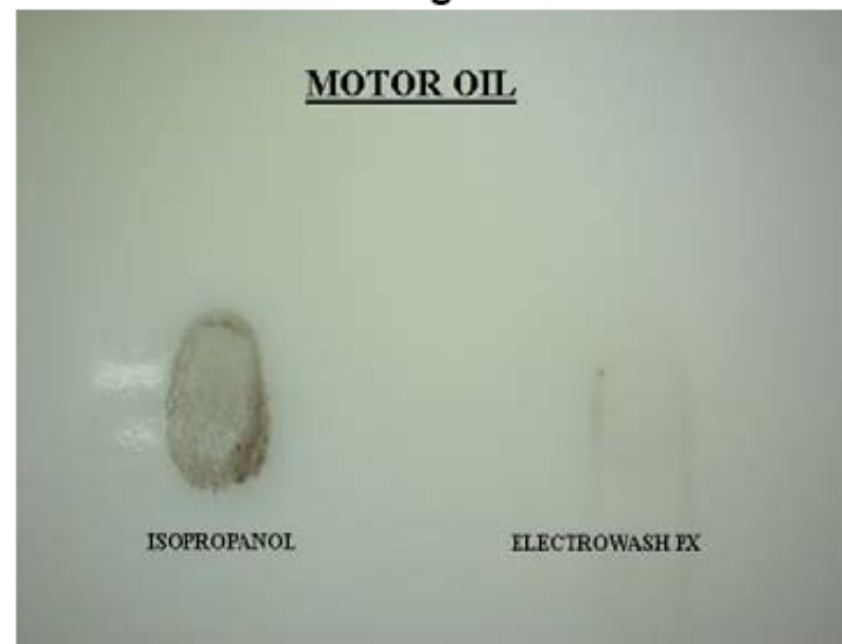
Soil after cleaning
