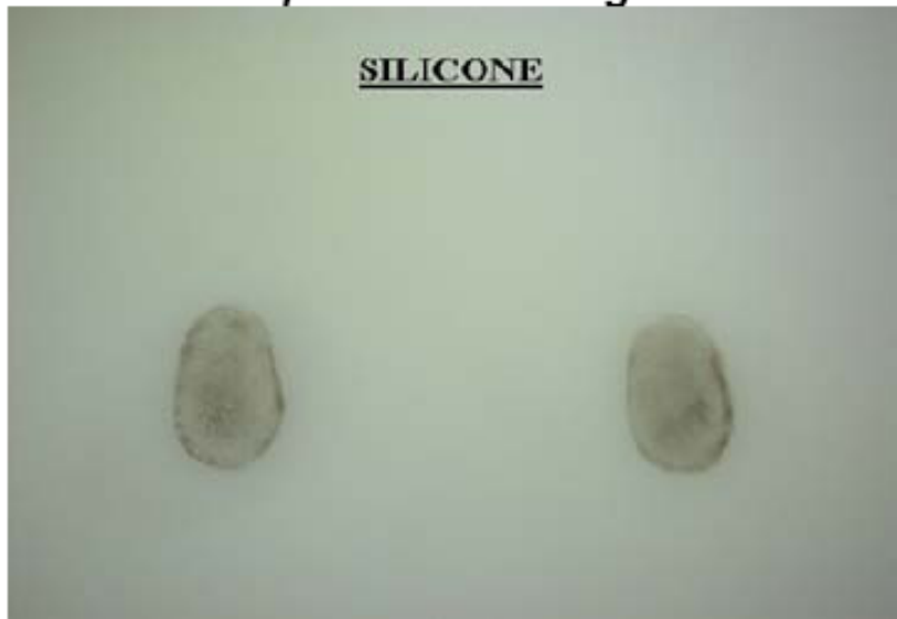
Soil prior to cleaning
