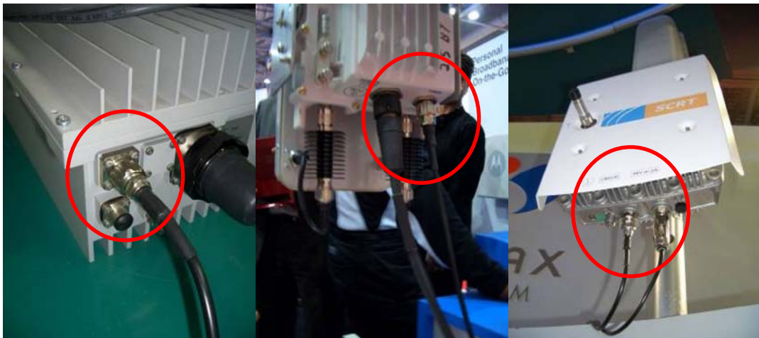
Figure 4: Examples of remote-radio heads with fiber optic links.
